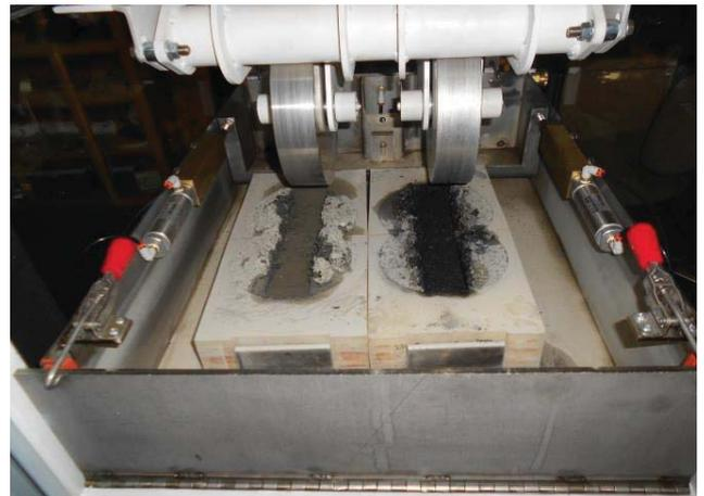
**Completed Hamburg Test with Gyrotory Samples**
