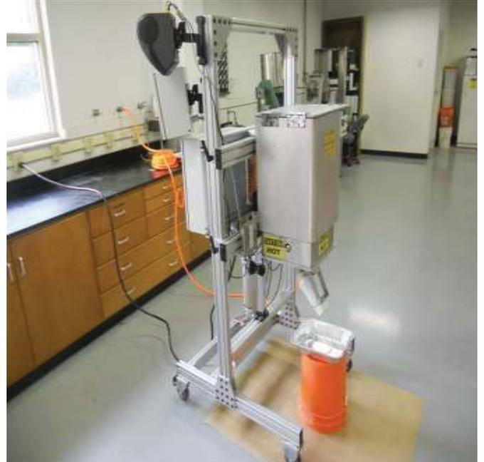
**"THE FOAMER"** is designed and manufactured to provide highly accurate and repeatable foamed asphalt samples that are used for Warm Mix Asphalt Mix Designs in the Laboratory. The Foamer can also be used for Cold Mix Designs and can be used as an Asphalt Dispenser. **"THE FOAMER"** is rugged and can easily be used in tandem with a laboratory mixer. Below are some features of **"THE FOAMER"**:
